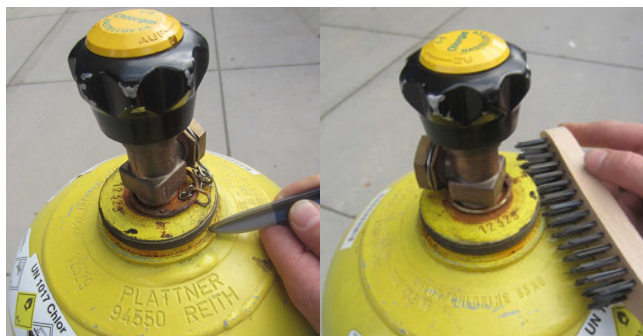
Fig. 1: Cleaning the thread and sealing surface
