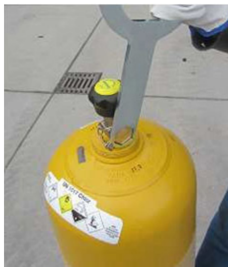
Fig. 3: Closing the emergency cap valve
